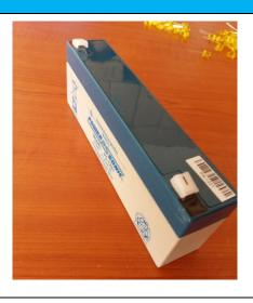
Sealed Lead Acid batteries of 1×12v \*18Ah, having desired life of 5 years.
