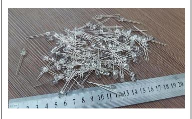
LED's are identified very well, amount of their desired life is 100.000 hours in lawful range for traffic light and traffic signals, and its light intensity is 8000mcd. Total numbers of LEDs in one device are equal to 507pcs for Seven Segment and emoji face.
