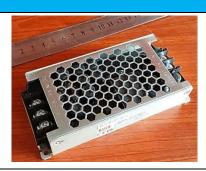
We used DC to DC converter for preparing of 5 volts from 12 volt to supplying LED display modules. This is manufactured by Meanwell company.
