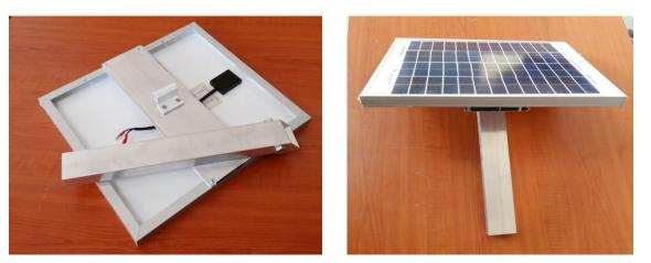
Solar panel is installed on pole by an aluminum tube. After orientation of solar panel into south, they are fastened by two house clips.
