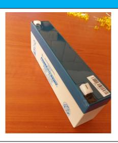
**Sealed Lead Acid batteries** of 2×12v 18Ah (36Ah), having desired life of 5 years.
