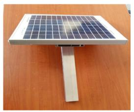
Solar panel is installed on pole by an aluminum tube. After orientation of solar panel into south, they are fastened by two house clips.
