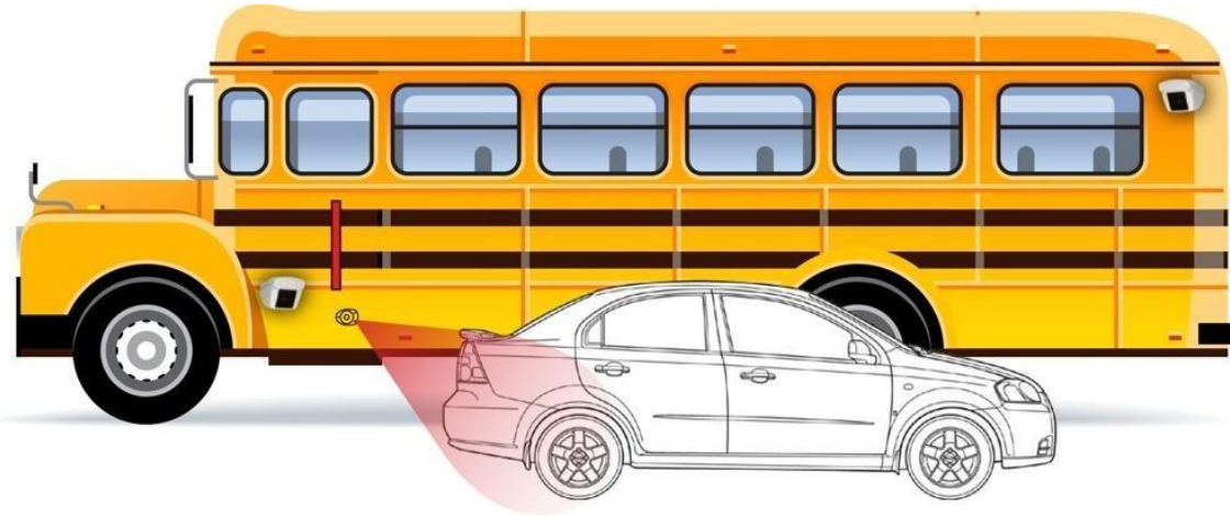
Picture 1: Stop Arm Violation Detector
