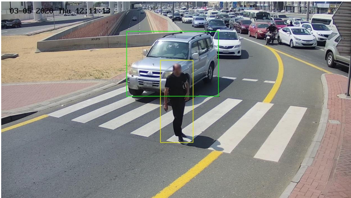
Picture 6: Sample of Pedestrian Crossing Violation on single Line
